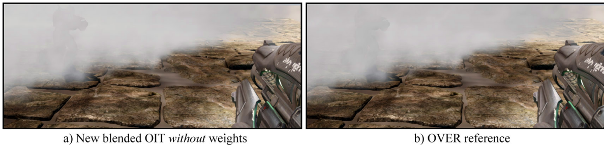
Figure 9. Smoke modeled as particles with similar color values. Left: new blended OIT without depth weights. Right: Sorted OVER reference image.
